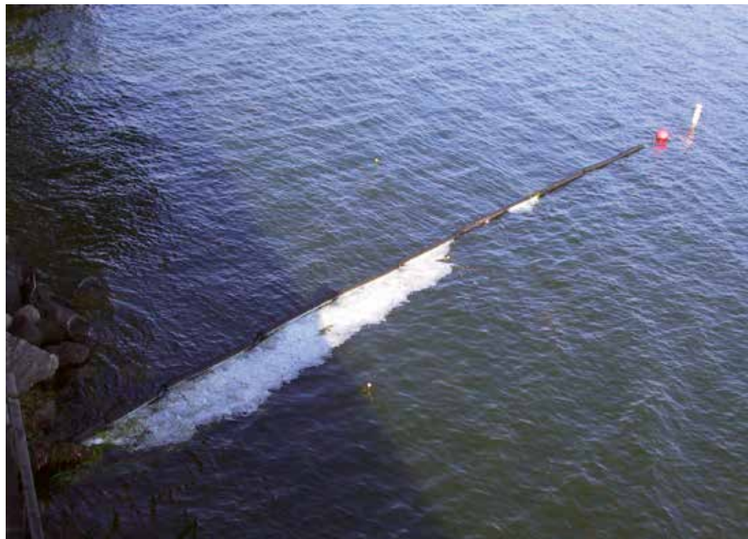
Figure 12. Floating material trapped on the single boom deployed at UW Center for Limnology in 2010 (photo: R. Lathrop, WDNR).
